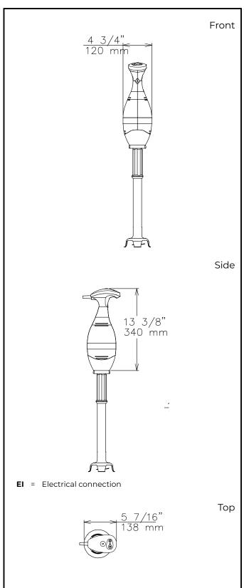
Electric Supply voltage: 602237 (DBP6565U) 110-120 V/1 ph/50/60 Hz **Total Watts:** 0.65 kW Plug type: USA NEMA 5-15P Key Information: External dimensions, Width: 5 7/16" (138 mm) External dimensions, Depth: 4 3/4" (120 mm) External dimensions, Height: 38 " (965 mm) **Shipping width:** 11 7/16" (290 mm) Shipping depth: 27 3/16" (690 mm) **Shipping height:** 7 1/16" (180 mm) **Shipping weight:** 13 lbs (5.7 kg)
